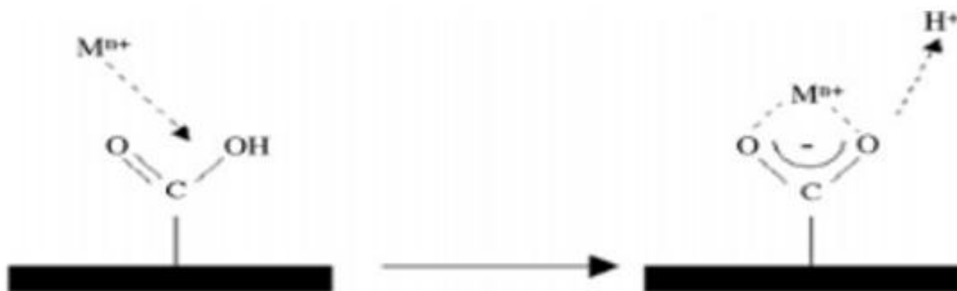
Figure 1. Cation Exchange Mechanism with the Carbon Surface Carboxylic Group (Yin et al. , 2007)
